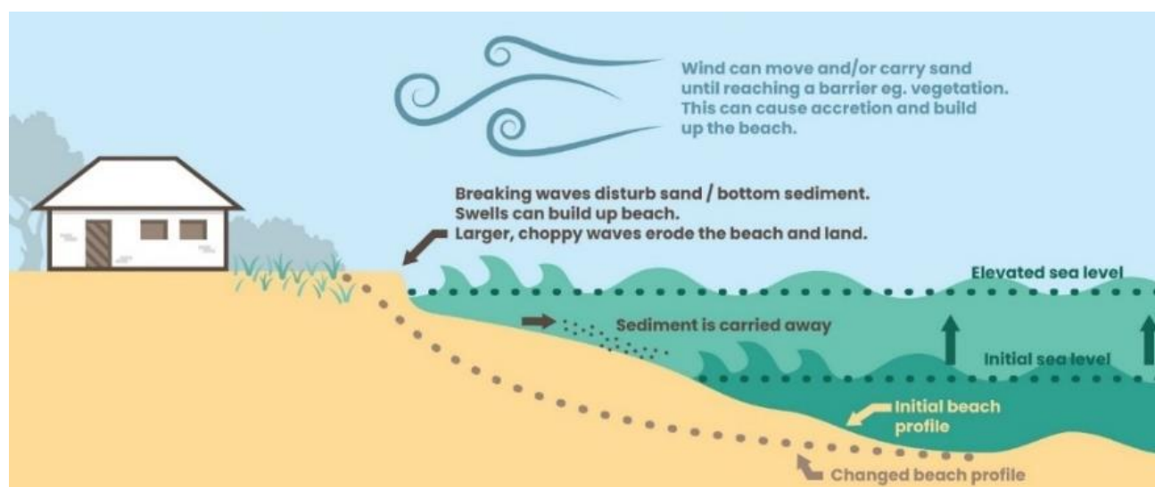
Figure 3. Process of coastal erosion and sea level rise
